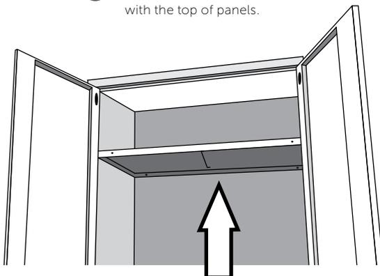
E Screw the top panel to the inside of the cabinet as indicated by the arrows.
