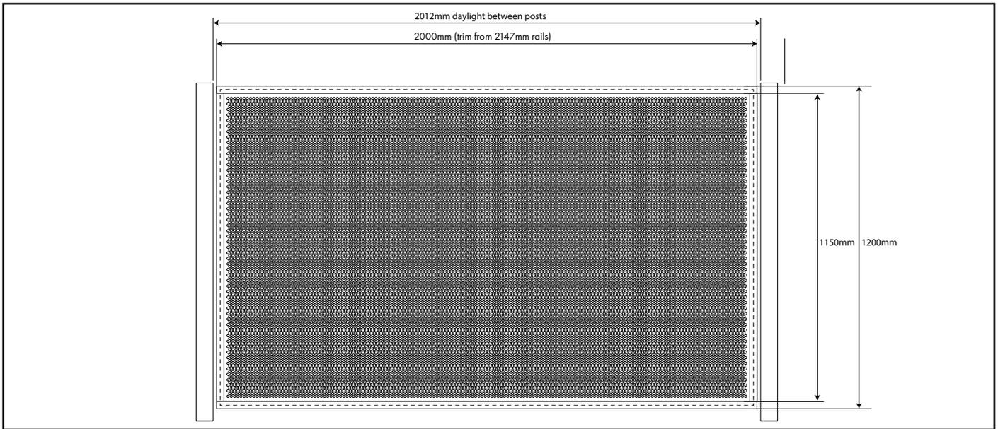
**NOTE** Assembled panels are standard at 2000mm wide x 1200mm high
